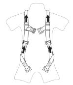
Individually adjust each shoulder strap (1) by pulling or releasing the slack end so that the sub-pelvic strap (8) is firmly in place under the buttocks.
