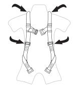
Slip on the shoulder straps (1) one at a time as if you were putting on a jacket. Be careful not to twist the straps.
