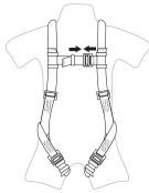
Attach the chest strap (2) parachute buckle and adjust the length so that the shoulder straps (1) are centered on each shoulder.
