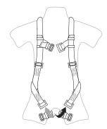
Pull each thigh strap (5) through the crotch and fasten the parachute buckles by passing the male buckle through the female. For tongue buckle insert the grommeted strap through the buckle. Fasten by inserting the tongue through the grommet. For quickconnect, insert male end into female end and apply pressure until the locking tabs snap into place. Ensure closure by checking tab positions in buckle window. Be careful not to cross or twist the straps.
